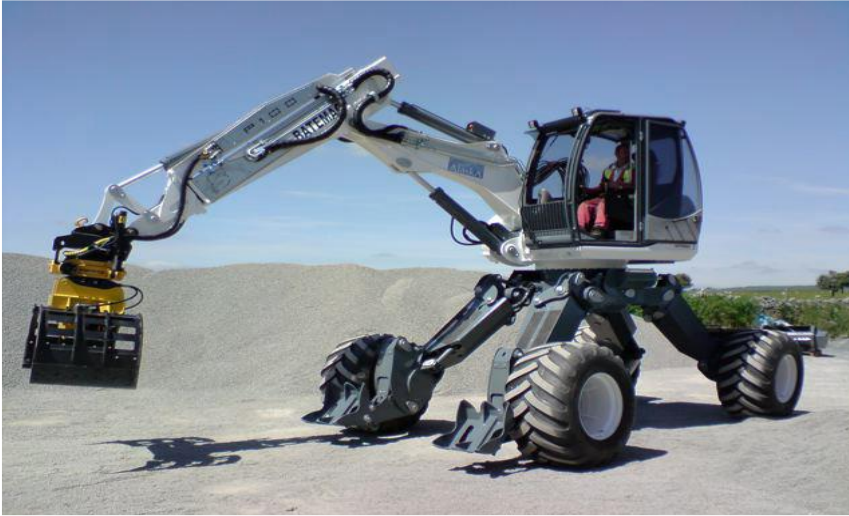
Machine raised into 'high' configuration (can work in up to 2m water depth)
