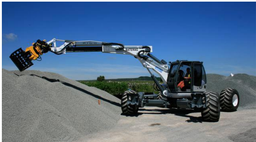
Machine raised into 'high' configuration (can work in up to 2m water depth)
