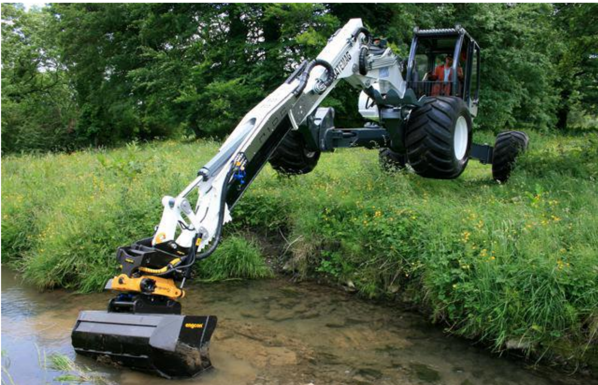
Ability to lift itself over sensitive bank edges – low ground pressure flotation tyres
